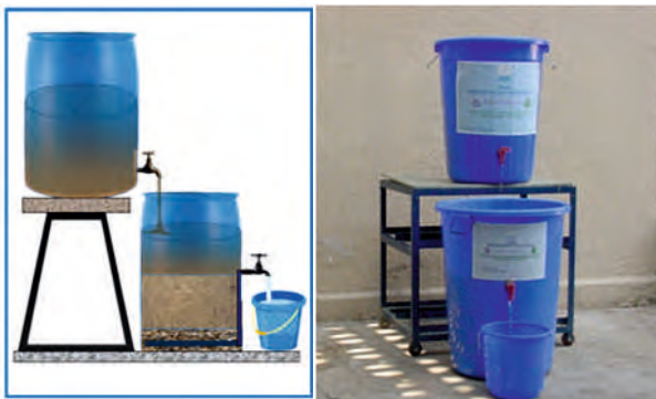
NEERI-ZAR Portable instant water filter
